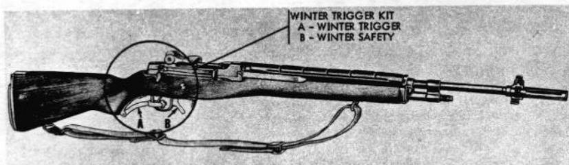
Figure 60. M14 rifle with winter trigger kit.
